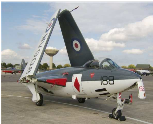
One of Britain's early attempts to build a carrier-borne fast jet; curved fuselage, but straight subsonic wing planform
