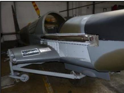
Powered by a Lycoming engine it carried a pilot in the front, and AEO + instruments in the rear cockpit. To minimise engine sound, the exhaust pipes ran inside noise attenuation ducts in the widened fuselage. It was very quiet and at 300 ft altitude virtually inaudible to the human ear. Three were built, but there was no series production.
