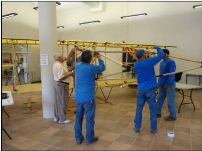
Disassembling a historic wood and fabric glider obviously brings with it the risk of 'collateral damage'; wood screws removed never go back as securely the second time and the builders were disinclined to allow any untu-
