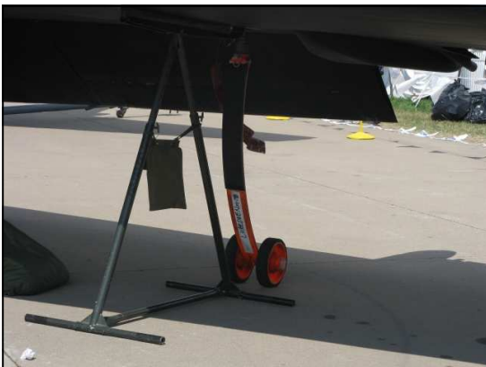
Lockheed TU-25 With a centre wheel only, when the aircraft lands the outrigger wheel is attached for taxiing.
